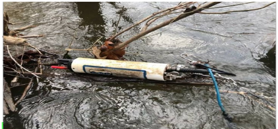
Picture of the LRSA water quality probe after serving an extended tour of duty in the Lehigh River basin. We were not able to safely retrieve the probe for four months due to historically long periods of historically high water conditions. Fortunately the probe still works even though it needs some refurbishment and R&R.
