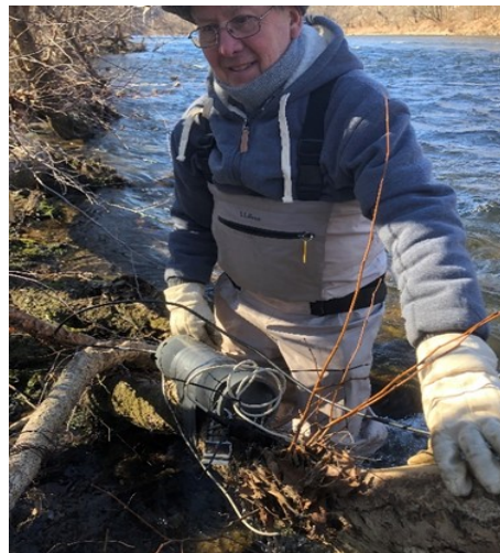
Figure 5 - The author at the site of the Hach DS5 WQ Probe deployment on the Lehigh River at Treichlers. Photo taken during probe maintenance in July 2018 (battery change and sensor calibration). The grey, cylindrical object on the tree is the cellular modem used to transfer data wirelessly from the probe to the Internet web site. Jim Deebel below right assists in probe deployment in March 2018.
