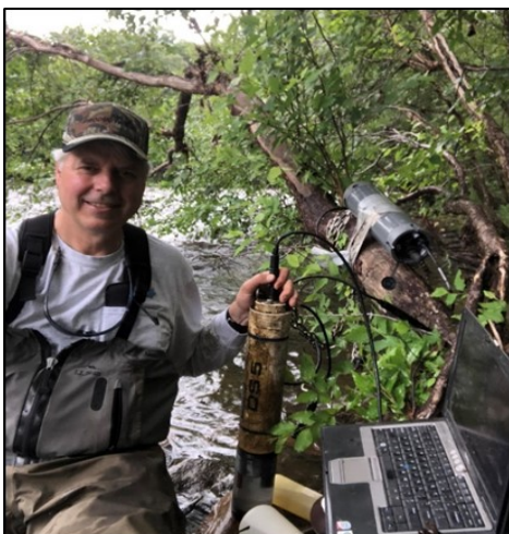
Figure 5 - The author at the site of the Hach DS5 WQ Probe deployment on the Lehigh River at Treichlers. Photo taken during probe maintenance in July 2018 (battery change and sensor calibration). The grey, cylindrical object on the tree is the cellular modem used to transfer data wirelessly from the probe to the Internet web site. Jim Deebel below right assists in probe deployment in March 2018.
